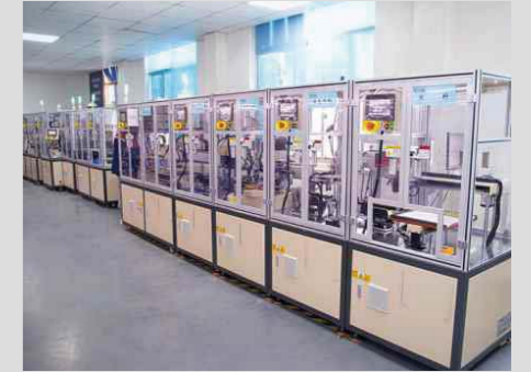
Transformer Automatic Assembling
